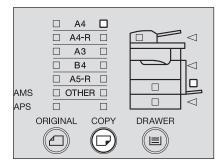
Press the media type setting button until the lamp of the media type placed on the bypass tray is lit.
